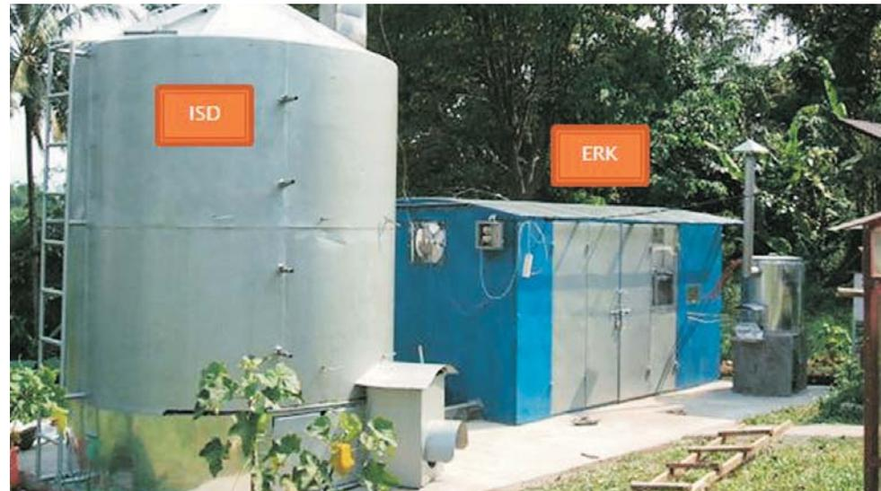
*This dryer works by combining the system of the Greenhouse Effect (ERK) and In-Store Dryer (ISD). Greenhouse effect works by utilizing recovered heat from the surrounding environment, while the In-Store Dryer is putting the seeds in place for further drying process so that the result is more even or uniform in dryness.*
