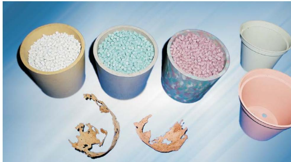
*This "green" plastic is a bio-degradable plastics formulated from emulsion of starch, natural rubber, polymethyl methacrylate, polyolefin, added with some filler materials and additives; through a radiation induced copolymerization by gamma irradiation.*
