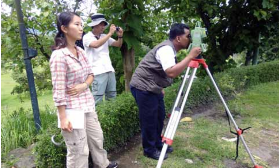
Using the Total Station to monitor the entire behavior of the stone structure and hill.
