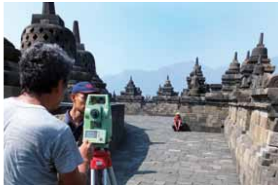
Using the Total Station to monitor the entire behavior of the stone structure and hill.
